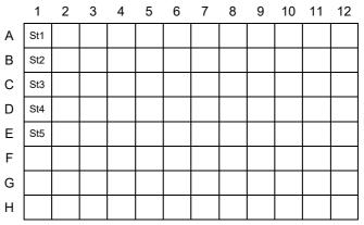
**Example plate layout** (example for a 5 point standard curve)
